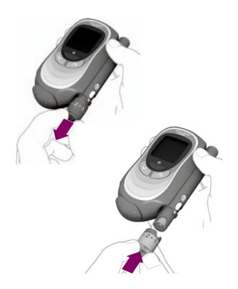
In the following description blood is obtained with the lancing device still attached to the meter. You can also detach the lancing device from the meter before using it to obtain blood.
