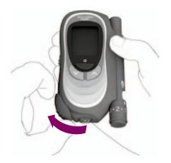
Start as for a blood glucose test: Either open the tip cover or select *Test* in the *Main menu*.
