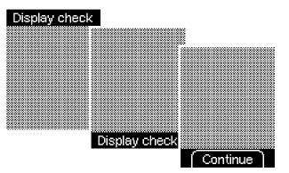
When you have closed the cassette compartment cover, the meter turns on again and runs the display check.
