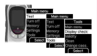
If you wish to check whether the display is working properly, in addition to turning on the meter, you can also do this via the display check in the *Tools* menu. In this case, the display check is shown until you cancel it (for no longer than 1 minute).
