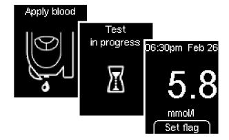
**2** Take your finger away from the test area as soon as *Test in progress* and the hourglass symbol appear on the display.
