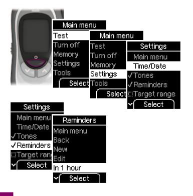
The meter can give you a one-time reminder to perform a test in 1 hour, 2 hours or 3 hours. You do not need to set a time for this. These reminders can be useful if you wish to check a result you just obtained, for example. When the reminder has been given, it is automatically deleted.
