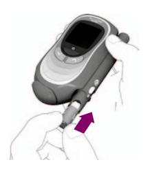
3 Insert the new lancet drum – white end first – into the lancing device.
