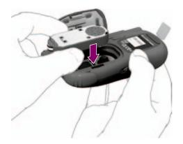
6 Insert the cassette in the meter with the silver side facing upwards.
