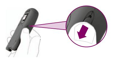
Push the release button for the cassette compartment cover in the direction of the arrow. The cover springs open.
