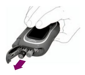
**3** Turn the meter so that the battery compartment faces downwards. The batteries fall out.
