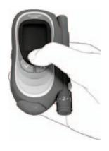
With the meter off, press and hold the On/Off button until the meter turns on (longer than 2 seconds).
