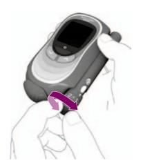
You can set the penetration depth of the lancet to 1 of 11 possible settings (0.5–5.5). The silver line (depth setting indicator) on the lancing device indicates the current penetration depth setting. The higher the number the deeper the penetration. The half settings for the penetration depth are indicated by a dot. The penetration depth 1.5 is set when the line points to the dot between 1 and 2.
