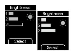
The more bars are filled in on the display, the brighter the display. The default setting is 2.
