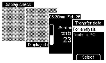
After the display check and the number of available tests, the *Transfer data* menu is displayed.
