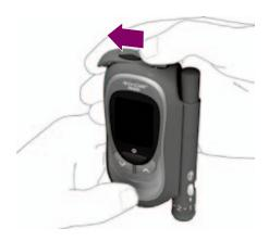
Push the battery compartment cover in the direction of the arrow as far as it will go to unlock it. You will have to overcome a slight resistance. The cover is properly unlocked when it slides over this resistance with a CLICK.
