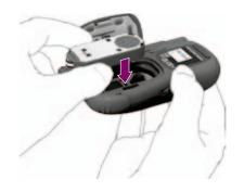
**15** Insert the cassette in the meter again with the silver side facing upwards.
