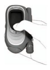
1 With the meter off, press and hold the On/Off button until the meter turns on (longer than 2 seconds).
