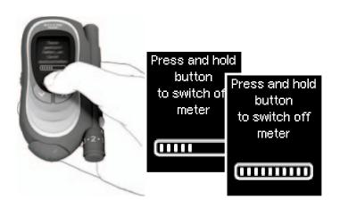
There are 2 different ways of turning off the meter: using the On/Off button or via the Main menu.
