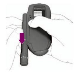
**2** Withdraw the lancing device by sliding it out in the direction of the arrow.
