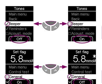
A checkmark  $\checkmark$  means that the function is activated. The command for the button is *Off* to allow you to deactivate the function.
