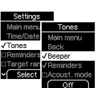
Beeper, Reminders and Acoustic mode can only be turned on and off. The procedure is always the same and is therefore only described here for Beeper.
