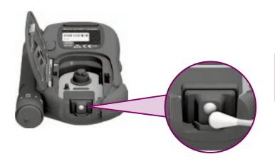
If the measuring optics are visibly soiled, clean the inside of the meter as follows:
