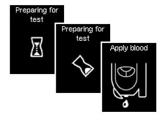
Then the meter will advance a test area to the tip of the cassette.
