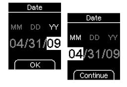
If the date you have set does not exist (e.g. April 31), the meter returns to the first setting position when you confirm the last entry with *OK* (step 7). You must correct the date before the meter will accept it.
