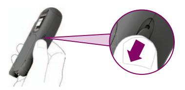
4 Push the release button for the cassette compartment cover in the direction of the arrow. The cover springs open.
