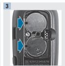
Slide the new batteries under the black tabs and button, with the (+) side facing up. Put the battery door back in place and snap it closed.
